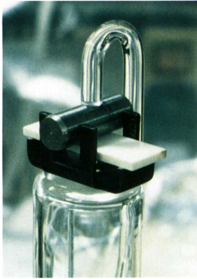
Plate 3 Three-point testing rig used to measure Young's modulus.
