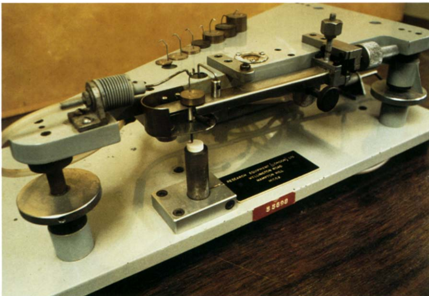
Plate 4 A pneumatic microindentation apparatus as used by Ridgway et al. (1970).
