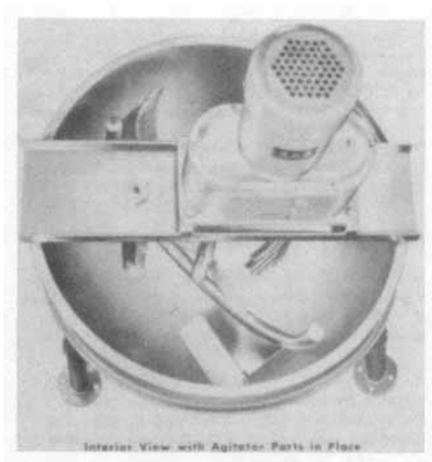
Fig. 14 Scraped-surface anchor agitator with auxiliary crossbar agitator. (From Ref. 20.)
