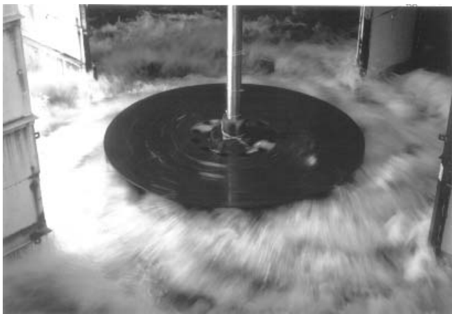
Figure 22-14 Aeration witness test in a 15 m square by 9 m deep tank.
