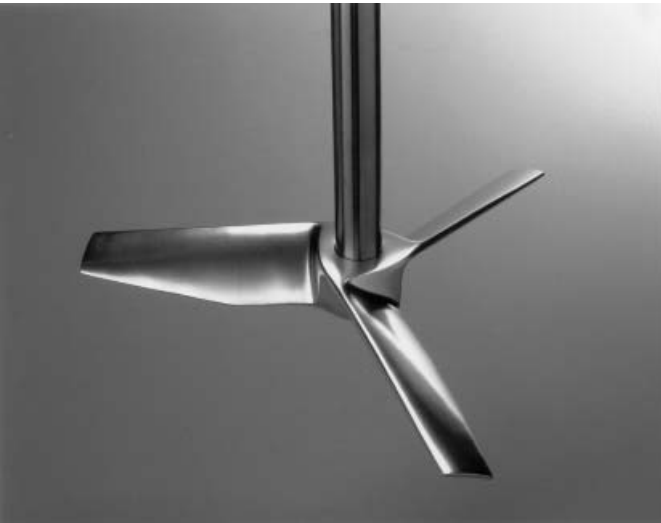
Figure 22-7 High efficiency flow impeller: N_p = 0.3 .
