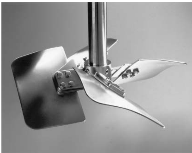
Figure 22-8 High solidity hydrofoil impeller for high viscosity or gas applications: N_p = 0.75 .
