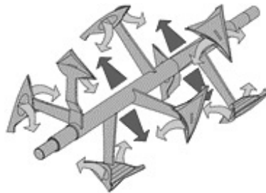
Figure 15-35 Plow mixer agitator and solids flow direction. (Courtesy of Kemutec.)
