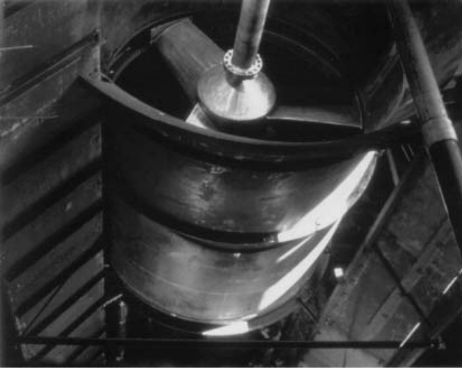
Figure 22-6 Full scale testing: a 3.2 m impeller in a 1 900 000 L test tank.
